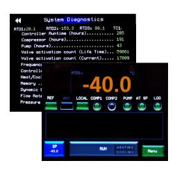
Programmable touch-screen controls with diagnostics and remote communications
