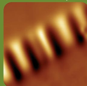
SHPM Image of NIST Calibration Sample, 77 K
