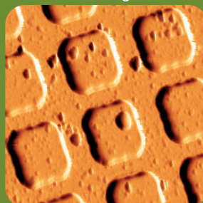
AFM (Phase) Image of Calibration Grating, 4.2 K
