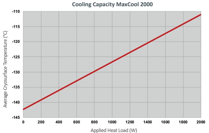
Single-circuit model; temperature shown is average of inlet and outlet temperature using typical cryocoil size; temperature difference between inlet and outlet at maximum load is typically 20°C; end point of curve is maximum load; performance at 50Hz can be 3- 5°C warmer than 60Hz performance shown; 25- 28°C cooling water.
