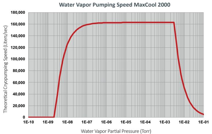
Single-circuit model; 2.4m refrigerant line; typical cryocoil surface area only; larger cryocoils will give greater pumping speeds and can be used in some applications; 25°C chamber temperature in line of sight with cryocoil; 60Hz; 25- 28°C cooling water.
