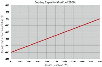
Single-circuit models; 25–28°C cooling water; temperature shown is average of inlet and outlet temperature using typical cryocoil size; temperature difference between inlet and outlet at maximum load is typically 20°C; end point of each curve is maximum load for that model; performance at 50Hz can be 3–5°C warmer than 60Hz performance shown.
